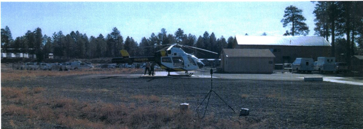
Figure 3. The sound system at 100 ft from the sound source. The sound level meter is taped to the top of the pelican case on the right of the tripod.
